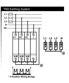
\* Connect N/ terminals together with wires or 3 Position Wiring Bridge
